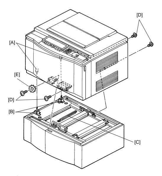
3. Place the copier on the paper feed unit aligning the positioning pins [A] of the copier with the positioning holes [B] of the paper feed unit.
